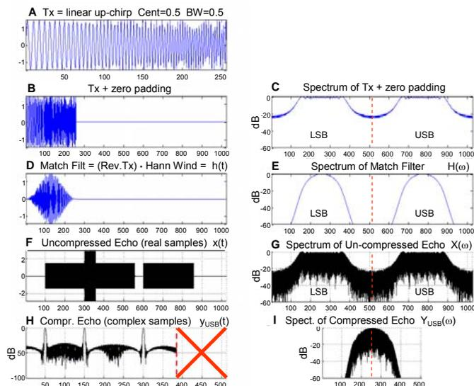
Figure 7 Matlab simulation of match filter and quadrature demodulator
