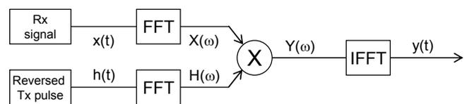
Figure 4 Match filtering in the frequency domain
