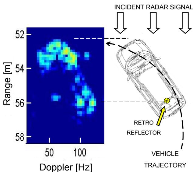
Figure 10 Geometry and radar results detailed plot
