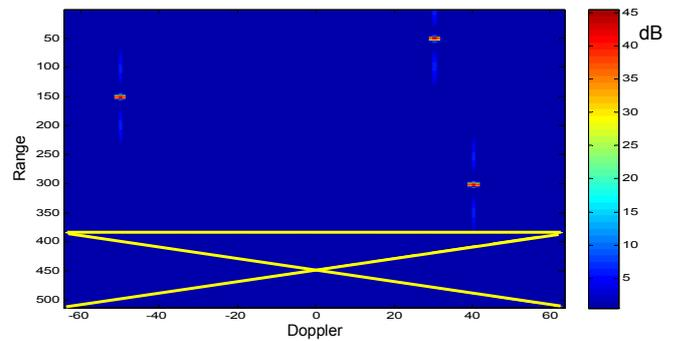
Figure 8 Range-Doppler image of the simulated data in Figure 7
