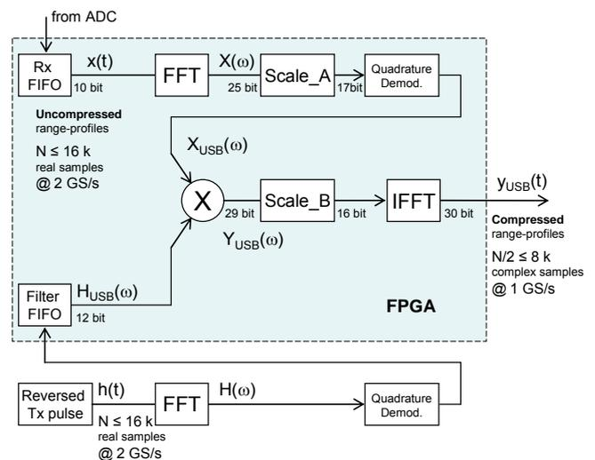
Figure 6 Combined match filter and quadrature demodulator
