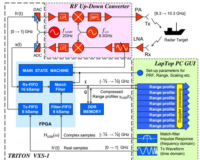
Figure 3 MuPuRF radar system functional block diagram
