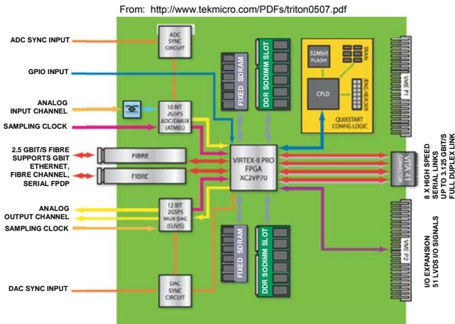
Figure 2 TRITON VXS-1 main components and signal paths
